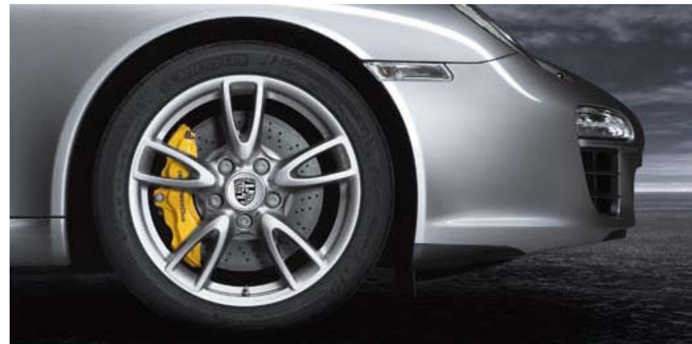
Porsche Ceramic Composite Brake (PCCB)
