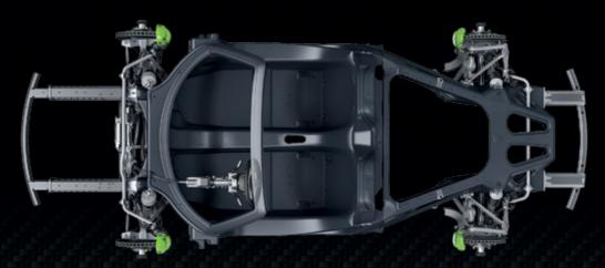
Monocoque and unit carrier
