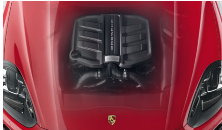
Cayenne GTS: 600 Nm between 1,600 and 5,000 rpm, 324 kW (440 hp) at 6,000 rpm
