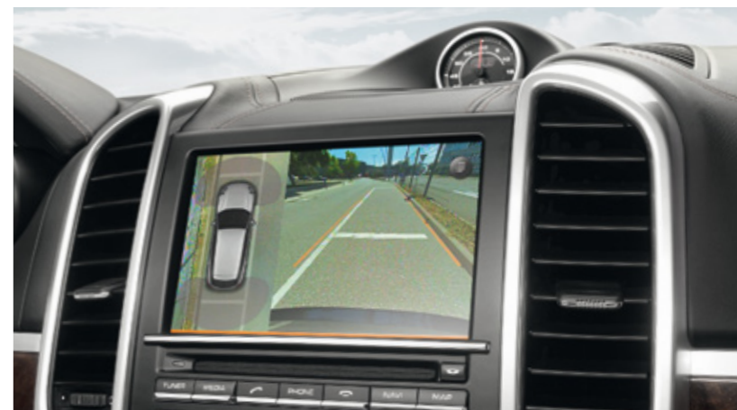
Surround View. Camera system for easier parking and manoeuvring (page 84).
