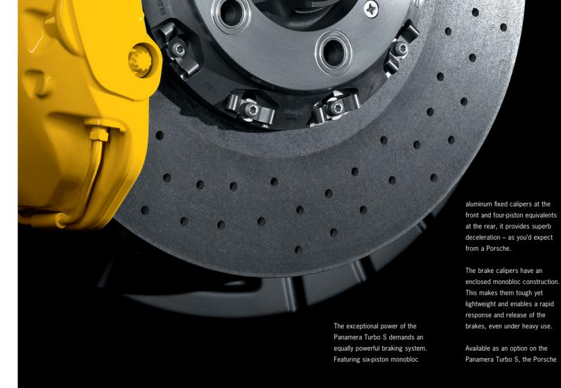
Ceramic Composite Brake (PCCB) has already proven its ability to cope with the harshest requirements of the racetrack.
