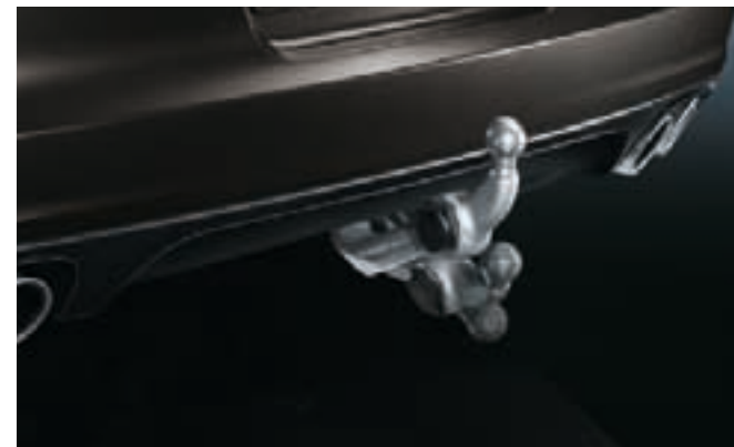
Electrically extending towbar system
