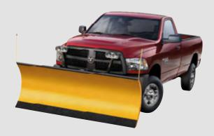
CAPABLE EFFICIENCY PUTS RAM IN FRONT. Extensive front axle developments in new Ram 3500 4x4 pickups start with a new front axle disconnect for increased efficiency. Front axles have also been enhanced for greater capability with new maximum front GAWRs; they're increased by 500 lb, raising maximum FGAWR to 6,000 lb.\* Further advantages include engineering that reduces parasitic losses and new lower viscosity lube that reduces resistance, both helping to enhance fuel efficiency.
