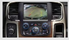
The new, large available 8.4-inch touch-screen radio in select new 2013 Ram Heavy Duty models now offers full-color displays, including three-dimensional imaging of landmarks and city modeling. New Active Grid Lines in the display are another Ram advantage — they're invaluable when backing up, changing with each steering wheel movement. Now you can easily and accurately align your hitch to the trailer, with no need to hop out to double-check, or bother with a spotter.
