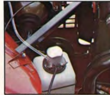
Large capacity windshield washer tank.
