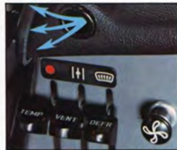
Ventilation and heating control levers.
