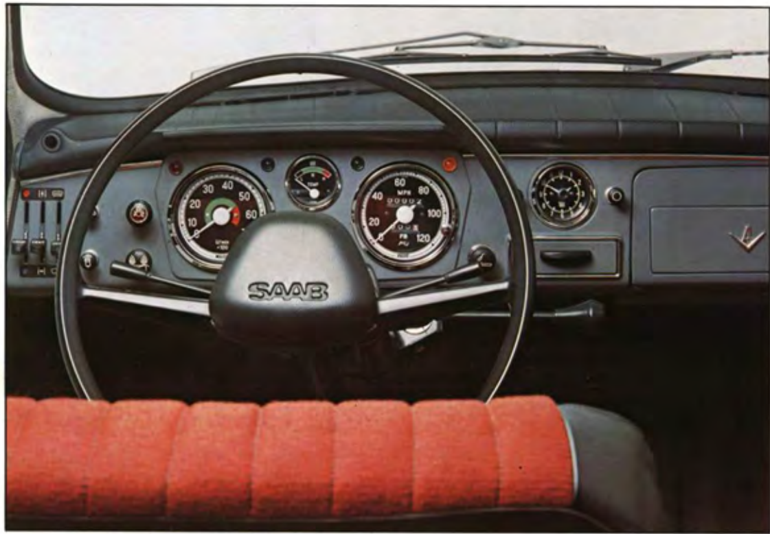
New steering wheel has padded hub for safety.
