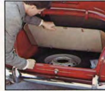
Spare wheel and tire in separate compartment.
