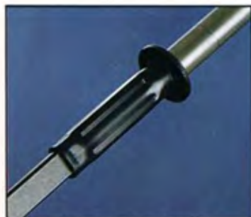
Collapsible steering column.
