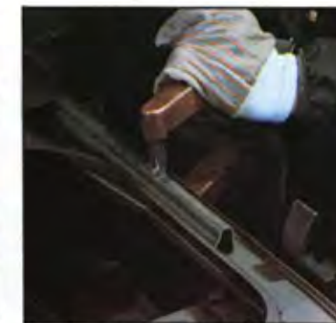
Steel sections in windshield pillars.
