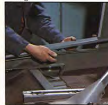
Brake lines are encased within steelplate.
