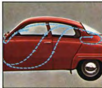
Air circulated through car and out rear.
