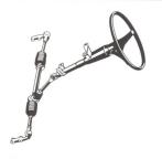
Rack and pinion type steering gear.
