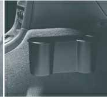
Waste/storage box – fitted on the passenger side of the centre tunnel. Can hold two soft-drink cans, five CD discs or a waste bag.
