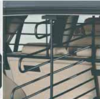
Cargo guard – metal guard that separates the passenger and luggage compartments. Gives the occupants added protection. (Wagon only)
