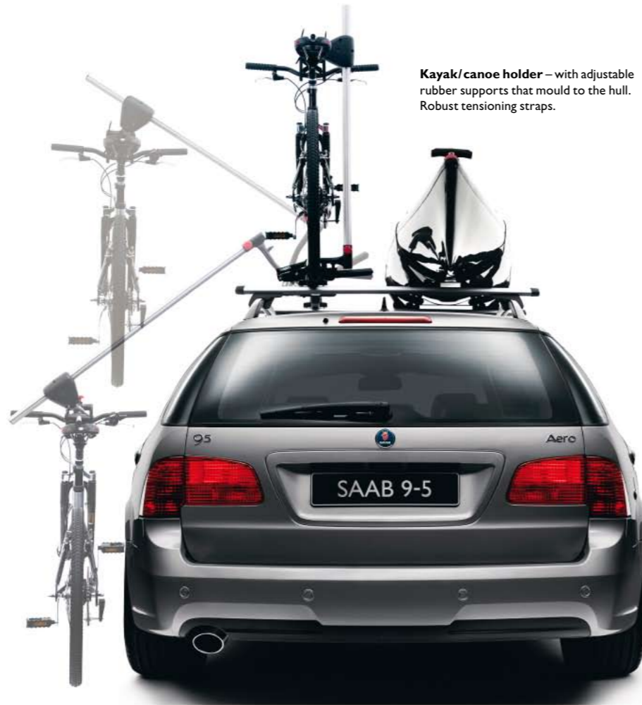
Bike holder with lift – the bike is inserted at door height, then lifted with the help of gas-filled struts and secured to the roof rack. Lockable. (SportCombi only)
