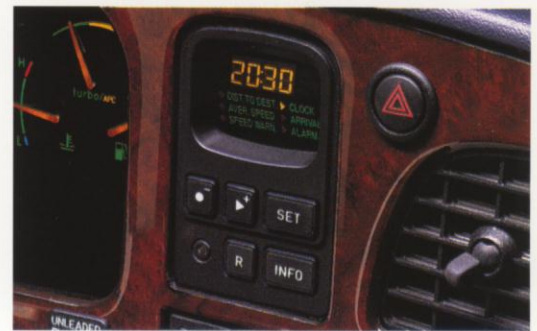
The Saab Car Computer (SCC) seen here in the optional walnut facia.
