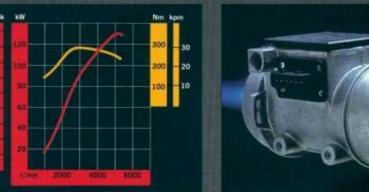
The Bosch LH-Jetronic fuel injection system ensures that the fuel/air mixture is always correct regardless of variations in climate or altitude.
