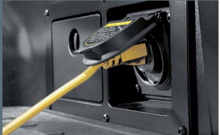
3 AVAILABLE 115V/400W DECK-MOUNTED AC POWER OUTLET
