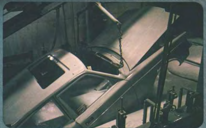
AFTER BEING SPRAYED WITH A ZINC-PHOSPHATE SOLUTION, THE BODY IS SUBMERGED INTO A PRIMER BATH.
