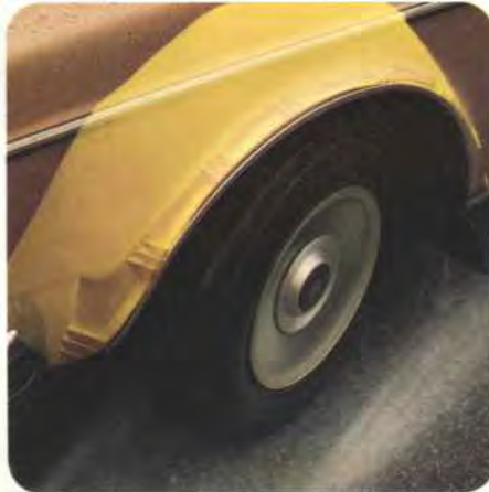
FRONT WHEEL HOUSINGS HAVE PLASTIC LINERS DESIGNED TO KEEP OUT ROAD DIRT AND SALT.
