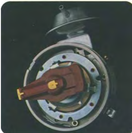
THE DISTRIBUTOR TRANSMITS HIGH VOLTAGE TO THE CORRECT SPARK PLUG.
