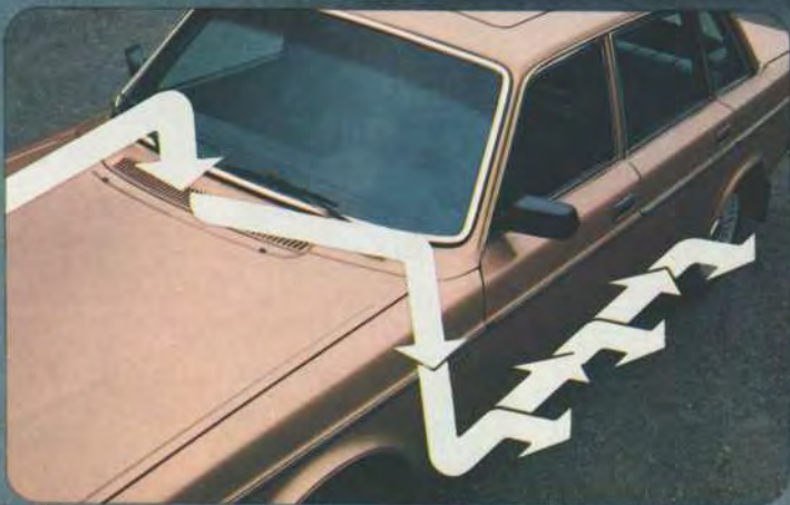
"SLIPSTREAM" VENTILATION HELPS KEEP MOISTURE FROM COLLECTING IN RUST-PRONE SPOTS SUCH AS DOOR SILLS.
