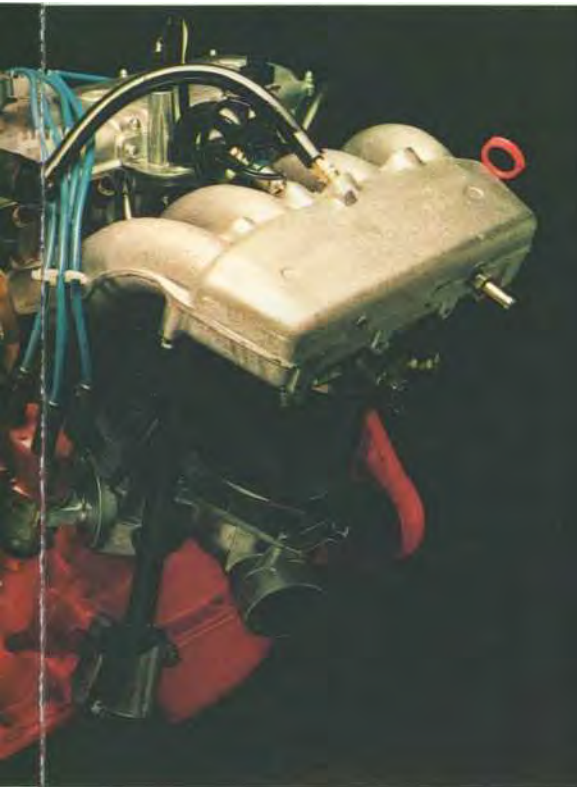
THE B21 F IS A 2.1 LITER IN-LINE FOUR WITH AN OVERHEAD CAM AND FUEL INJECTION.
