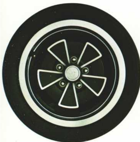
5" steel rims. Cast aluminium "mag" type hubs. 165 HR 15 radial ply tyres.
