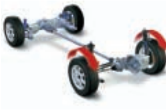
If you are cruising on straight, dry roads, the car is almost entirely front-wheel driven for optimum stability and fuel economy.
