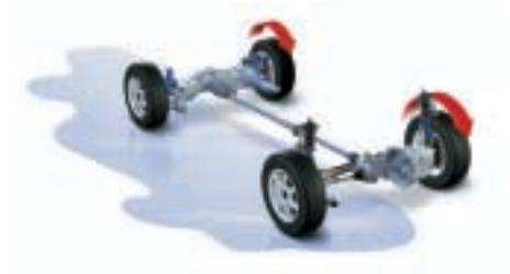
If one or both wheels spin on one side of the car, more power goes instantly to the ones with the best traction.
