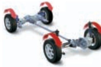
If the front wheels show any tendency to spin, the AWD system responds instantly by redistributing up to 50% of the drive to the rear wheels for maximum traction and stability.
