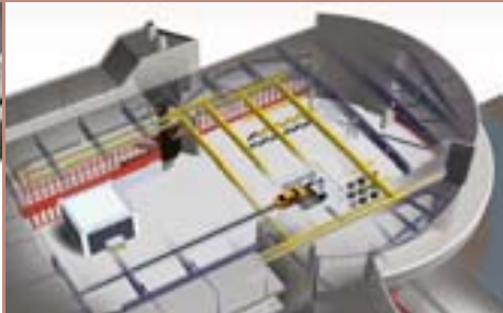
Within the center, our 850-ton barrier can be positioned and configured to replicate the dangers of countless real-life traffic situations. What's more, this is where collisions take place between a vehicle entering the center through the fixed tunnel and another entering from a pre-defined angle via the movable test track.
