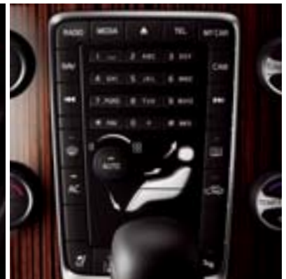
Electronic Climate Control (ECC)
