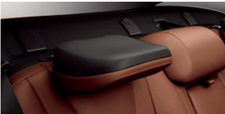
Power foldable rear head restraints
