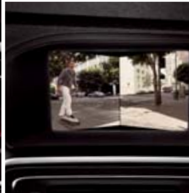
Front Blind View Camera
