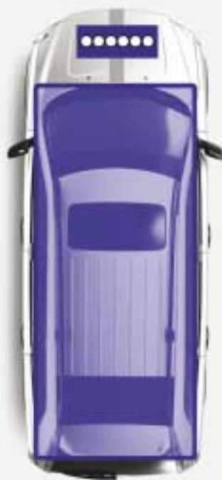
XC90 Transversely mounted engine creates maximum interior space.
