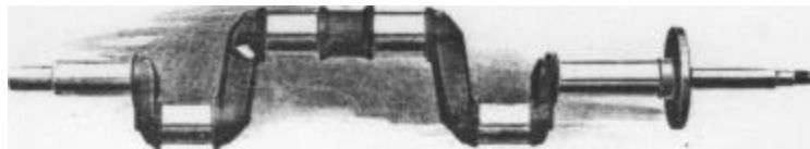
The Hudson crank shaft is a one-piece, heat treated drop forging. Each one tested to a tensile strength of 100,000 pounds. Forged under the most exacting specifications.
