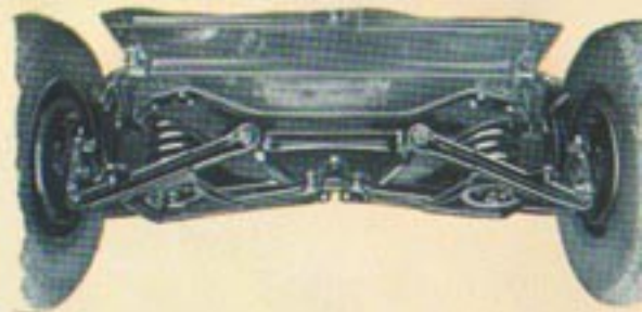
Coil springs in front and leaf springs in rear . . . finest combination known for easy riding and stability.
