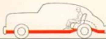
Conventional Cars Riding over rear axle and above frame, reduced headroom and comfort.
