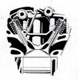
The engine "breathes" easily . . . fuel-air mixture travels down-hill from carburetor, through intake manifold, into combustion chamber. After combustion, gases continue downhill through exhaust manifold.
