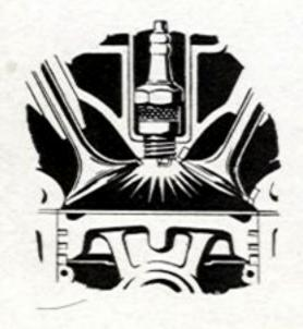
They're dome-shaped ... with centered spark plugs and big, laterally-placed valves. This achieves short flame travel ... quicker, more complete combustion ... reduces loss of heat energy through chamber surface.
