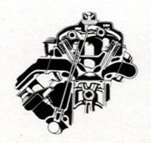
Lateral placement allows big valves with high lift and direct-flow porting. Noiseless hydraulic tappets give actuation through new arrangement of push rods and rocker arms with twin rocker shafts.
