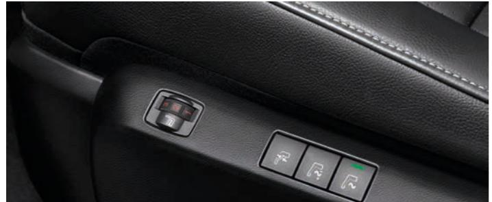
Tilt and height-adjustable driver's seat and front passenger's seat
