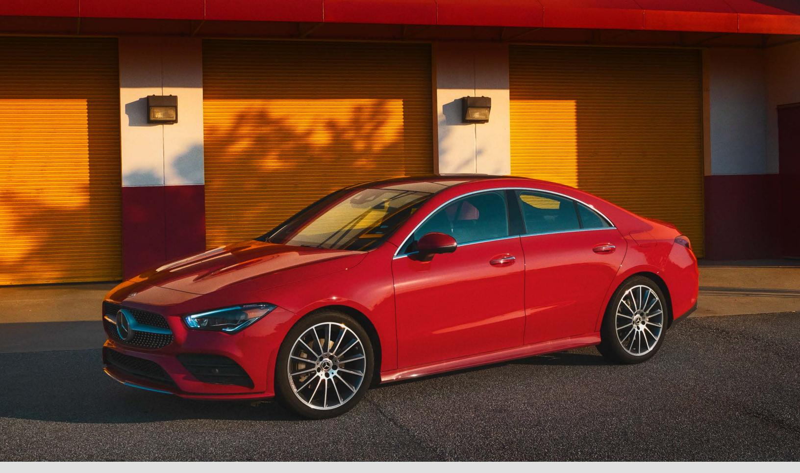
CLA 250 Coupe SPECIFICATIONS /ENGINE 2.0L inline-4 turbo TRANS 7G-DCT 7-speed auto /POWER 221 hp @ 5,500 rpm /0-60 MPH  $\rightarrow$  6.3 sec<sup>14</sup> /DRIVE Front-wheel or 4MATIC® all-wheel WHEELS 18" multispoke
