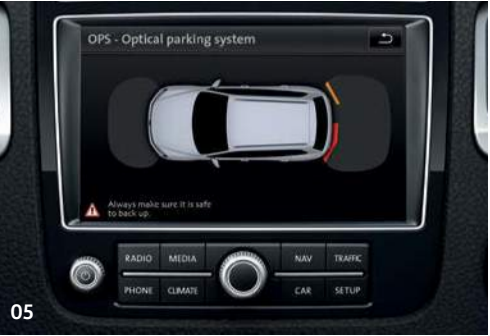
05 Parking sensors, ultrasonic front and rear alert you with an optical and audible warning as soon as your vehicle approaches an object to the front or rear when manoeuvring into a parking space. A visual representation of how close the front or rear of the vehicle is to an object will also be displayed on the vehicle's infotainment system display. Standard on all models.
