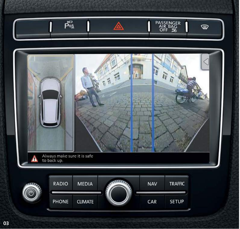
03 Area view's front, rear and side cameras provide a 360 degree exterior view around your Touareg transmitted to the RNS 850 Connect touch-screen navigation/DAB infotainment system's display, providing a bird's-eye view to the front and enabling you to see around left and right hand corners to an angle of over 90 degrees. Standard on R-Line Plus models and optional on all other models.
