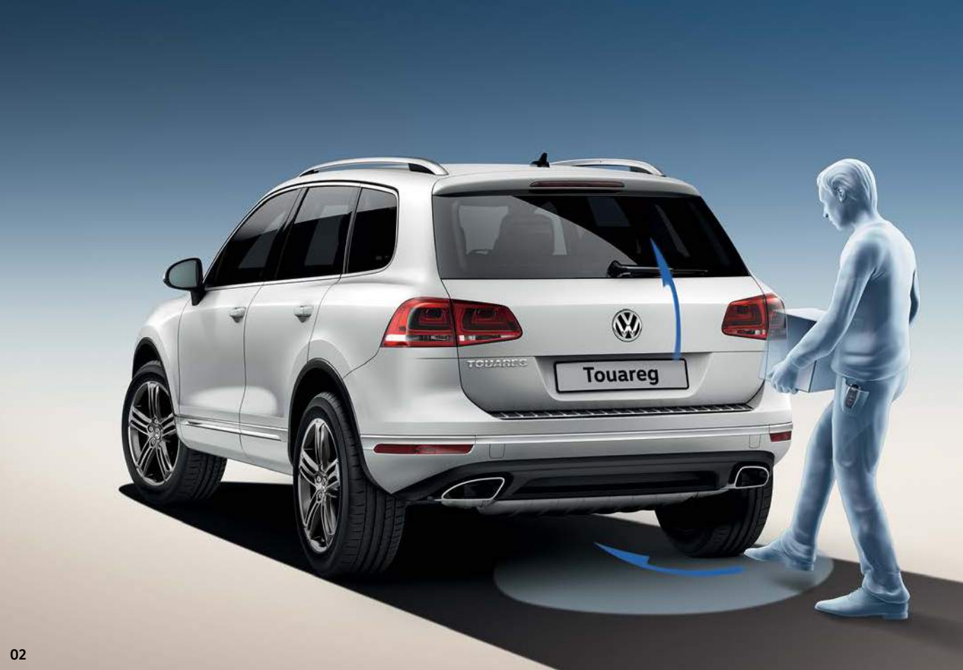
02 The hands free tailgate opening function enables you to open the tailgate without having to make contact with your Touareg as long as you have the key in your possession. A small foot movement triggers sensors at the vehicle's rear and the rear tailgate will open out. Hands free tailgate opening is a function that is part of the keyless entry/keyless start and full electric tailgate operation option on SE models only.
